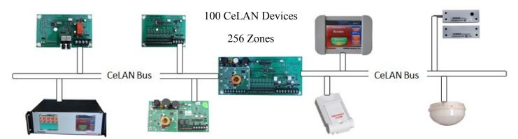
**Panel Data Bus**: CeLAN - 128 Bit AES Encrypted, two electrically independent, CeLAN data buses with a maximum of 100 devices total.
