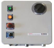
Several configurations available, assembled in a ready to install professionally labeled 12 x 12 NEMA 4 enclosure with standard or lighted open, close, and stop button options as well auto/manual selector and system disconnect.
