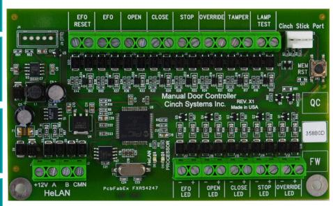
Supports bidirectional HeLAN communications. This exclusive technology surpasses ladder logic wiring methods eliminating wiring errors between the controllers for minimal installation time providing added value to turnkey installations.
