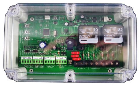
Provides individual LED indicators on each input and relay output for dynamic display of system functions.
